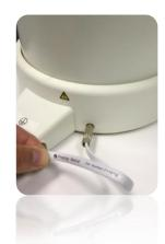
Insert the supplied 3,5mm jack plug from the printer into the rear of the autoclave as shown in the image below.
